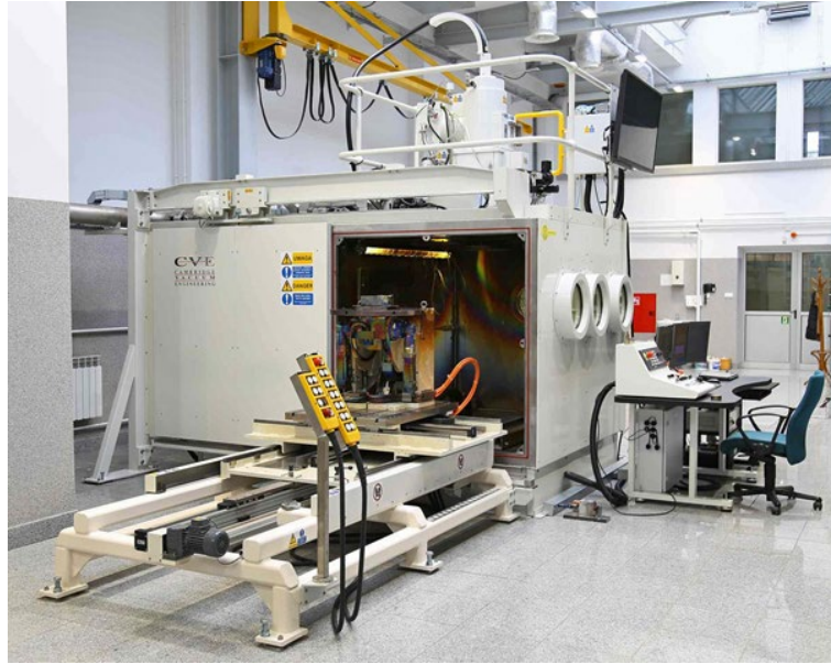
Figure 4. CVE EB756 model XW150:30 electron welding machine
